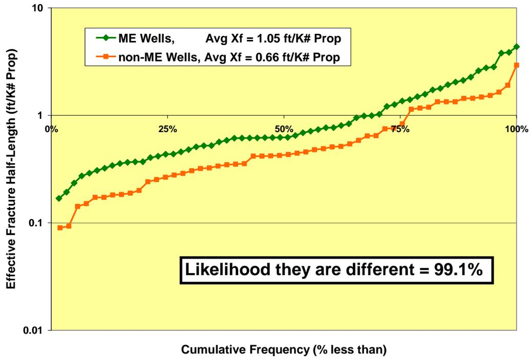
Fig. 2. Cumulative Frequency Histogram of Proppant Weight normalized effective fracture half-length for the 61 ME wells compared to the 53 non-ME wells.
