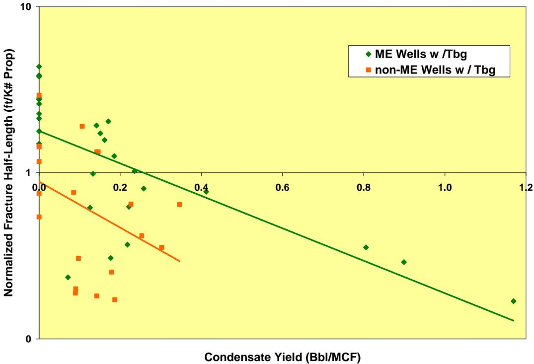
Fig. 6. Proppant weight normalized effective fracture half-length for the 27 ME and 20 non-ME wells with tubing installed as a function of condensate yield.
