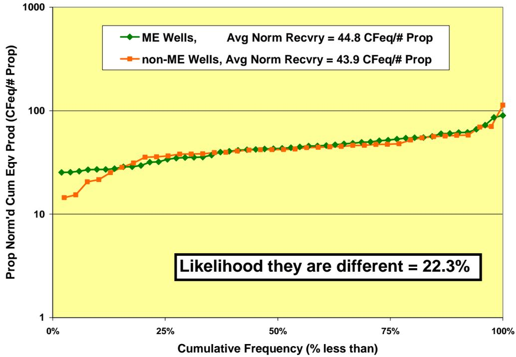
Fig. 3. Cumulative Frequency Histogram of cumulative equivalent gas production normalized for weight of proppant placed in the 61 ME wells and 53 non-ME wells.
