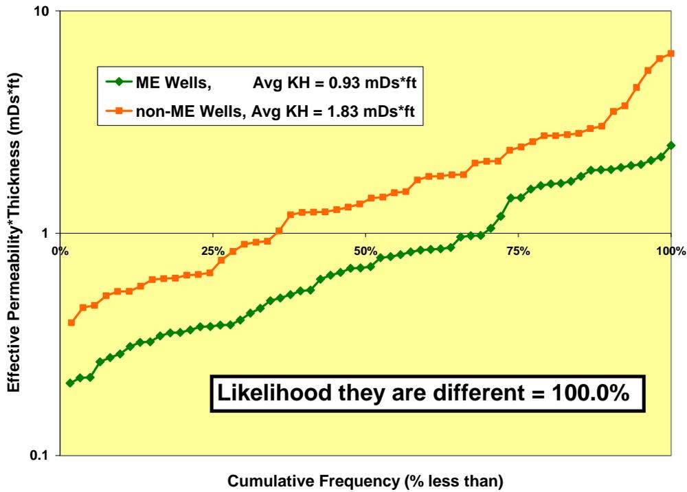
Fig. 1. Cumulative Frequency Histogram comparing reservoir quality (permeability \* thickness) of the 61 wells with ME versus the 53 non-ME wells.
