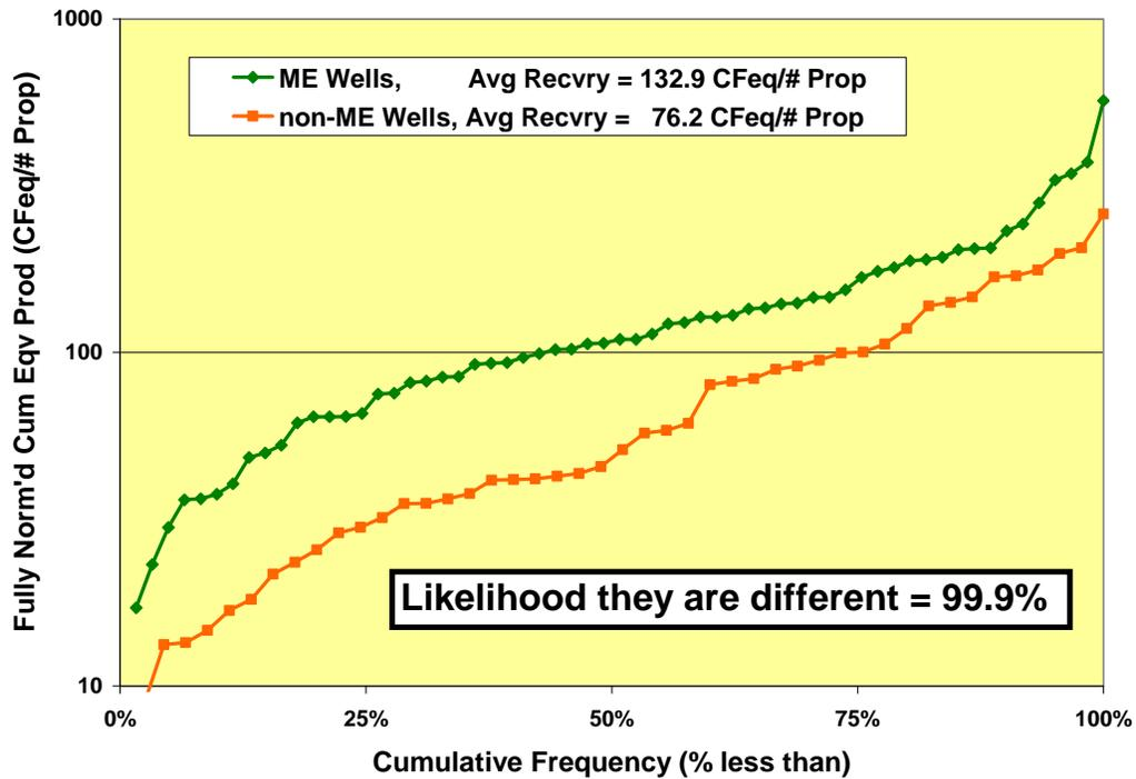
Fig. 4. Cumulative Frequency Histogram of 30 day cumulative equivalent gas production normalized for time on production, reservoir quality, amount of pressure drawdown and weight of placed proppant for 61 ME wells and 53 non-ME wells.
