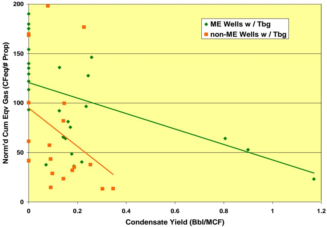
Fig. 5. 30 Day Cumulative Equivalent Gas Production normalized for time on production, reservoir quality, pressure drawdown and placed proppant as a function of condensate yield for the 27 ME wells and 20 non-ME wells with tubing.
