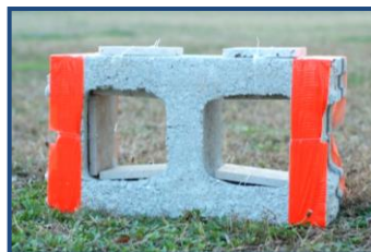
Above: Concrete block with travertine tiles attached.
