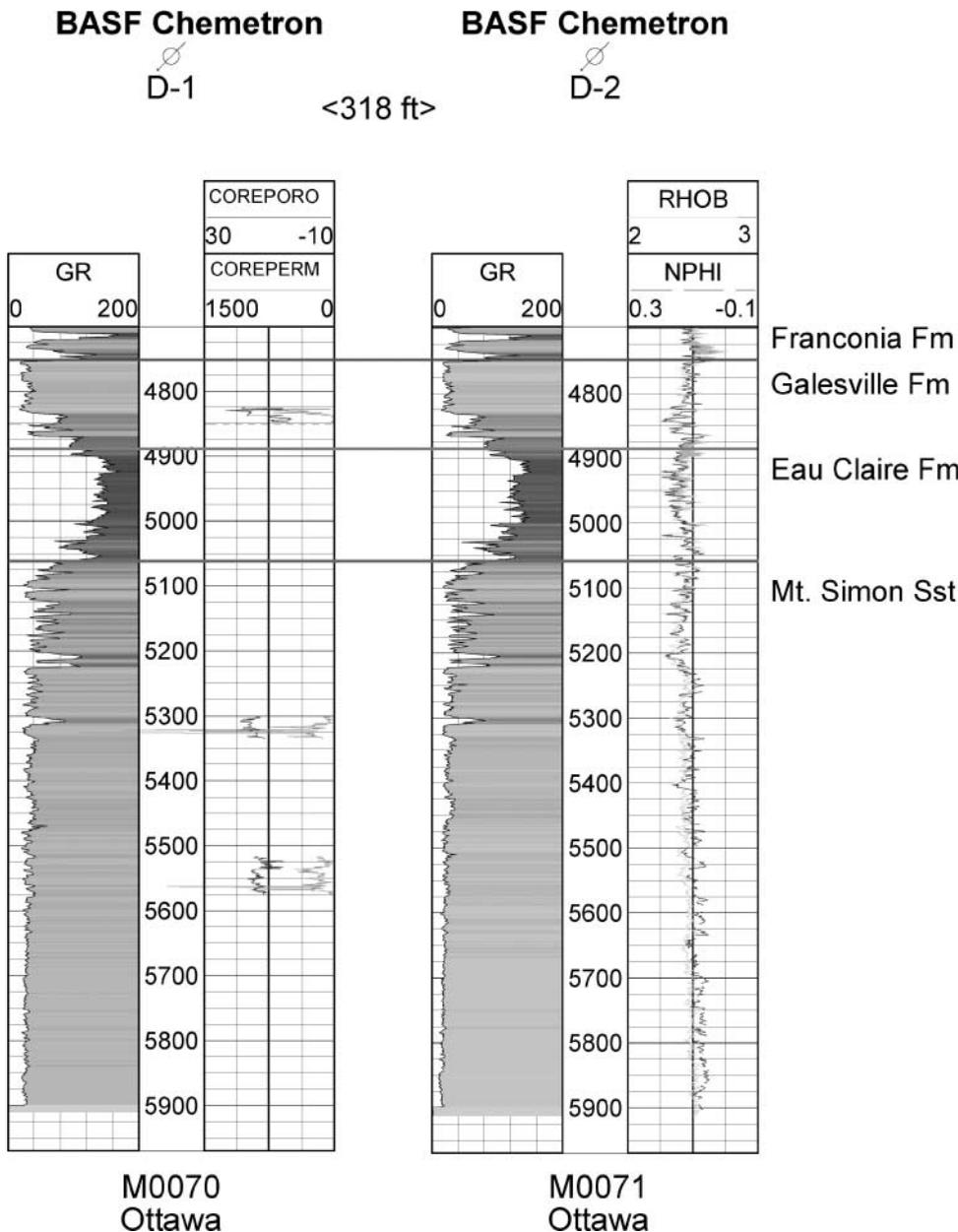
**Figure 6.** Key Mount Simon wells near Holland, Ottawa County, southwestern Michigan. Well logs show gamma-ray (GR) logs on the left track. The right log track in the D-1 well shows conventional core porosity (%), COREPORO) and permeability (md, COREPERM). The right track in the D-2 well is the bulk density (gray, RHOB) and neutron porosity (black, NPHI).
