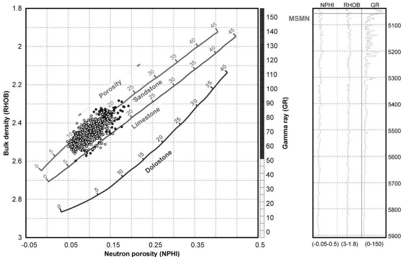
**Figure 8.** The NPHI-RHOB log crossplot from the BASF Chemetron D-2 well showing the interpreted porous sandstone lithology in the Mount Simon Sandstone.
