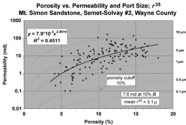
**Figure 12.** Plot of conventional core porosity versus permeability for Mount Simon Sandstone samples in the Semet-Solvay #2 well, Wayne County, Michigan.
