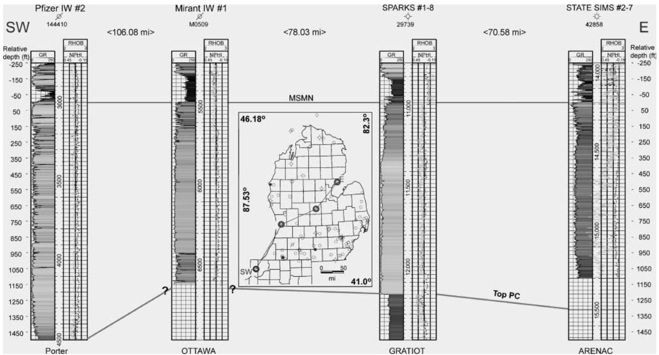
**Figure 5.** Southwest to northeast stratigraphic cross sections showing logs from complete or near complete penetrations of the Mount Simon Sandstone. MSMN = top Mount Simon Sandstone; Top PC = top Precambrian. Note that bulk density (RHOB) and neutron porosity (NPHI) logs in some wells are of questionable reliability, especially in deeper well penetrations (see Sparks #1-8 and State Simms #2-27 wells). GR = gamma ray.
