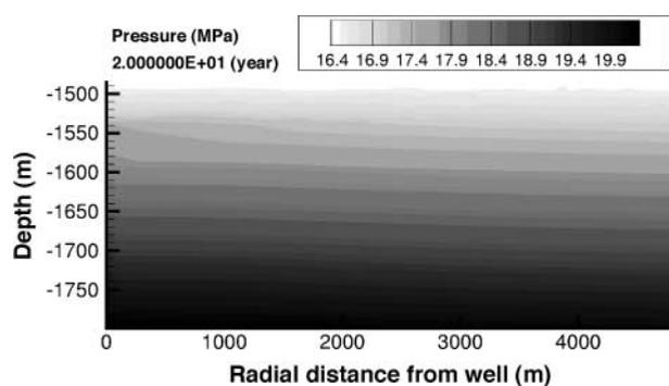
**Figure 23.** Formation pressure in the Mount Simon Formation after supercritical CO<sub>2</sub> injection.
