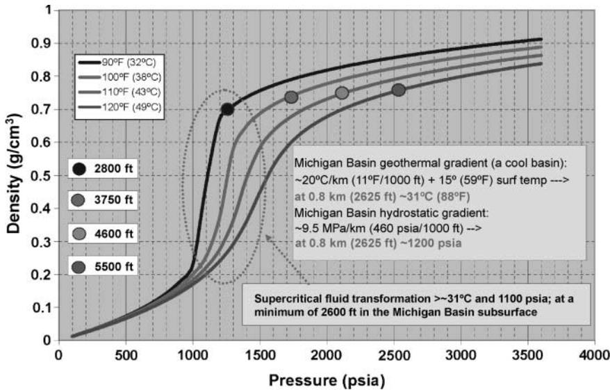
**Figure 1.** Pressure-temperature-density plot for CO<sub>2</sub> and pressure-temperature-depth relationships in the Michigan Basin. Colored dots represent the pressure-temperature-density relationships at selected depths in the basin.
