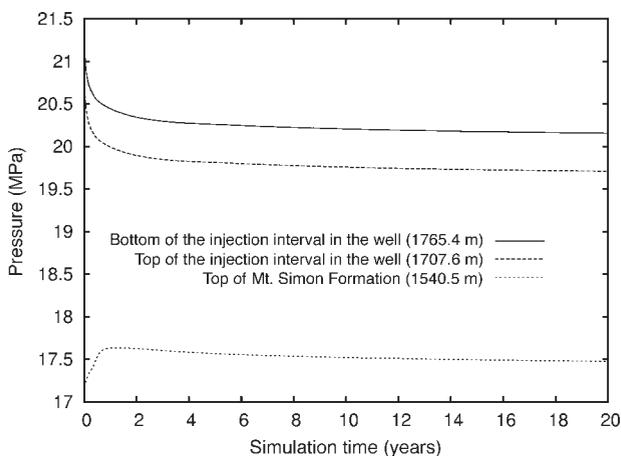
**Figure 18.** Injection well pressure during CO<sub>2</sub> injection into the Mount Simon Formation at a rate of 600,000 t/yr.
