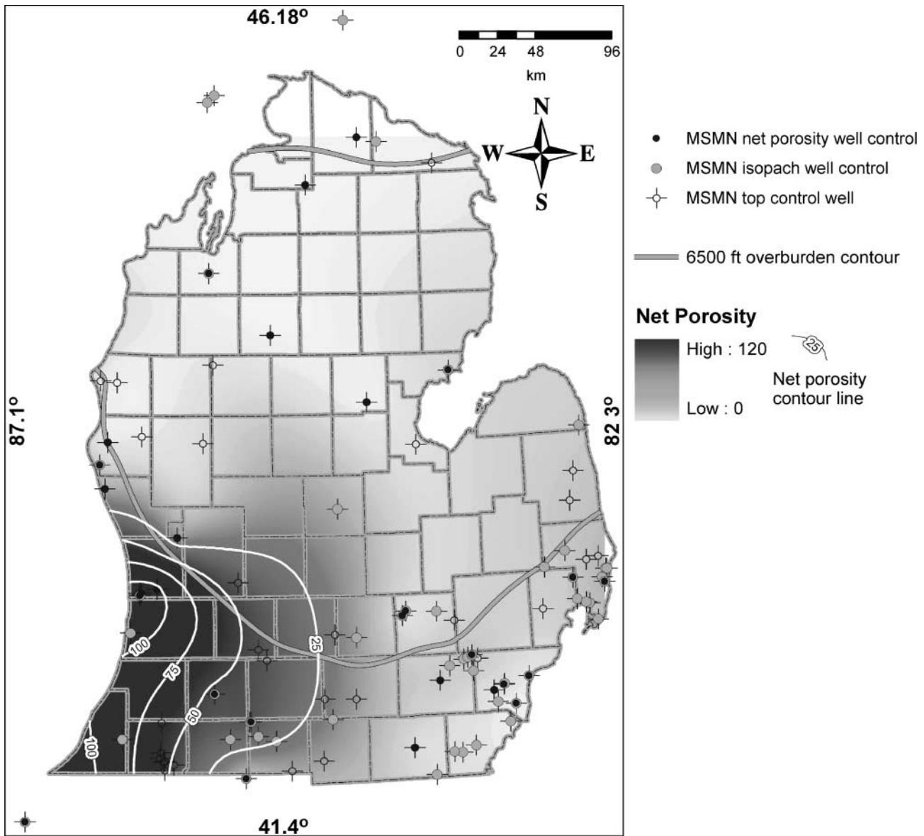
**Figure 13.** Gridded and contoured net porosity for the Mount Simon Sandstone in Michigan. Geostatistical analysis was done using ordinary kriging and a spherical variogram model with a root-mean-square error for 32 data points of 23. MSMN = Mount Simon Sandstone.
