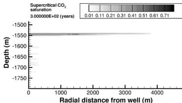
**Figure 22.** Saturation of supercritical CO<sub>2</sub>, 280 yr after the end of the 20-yr injection into the Mount Simon Formation.
