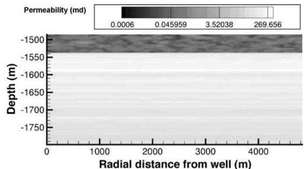
**Figure 16.** Geostatistical realization of intrinsic permeability in the Mount Simon and Eau Claire formations.
