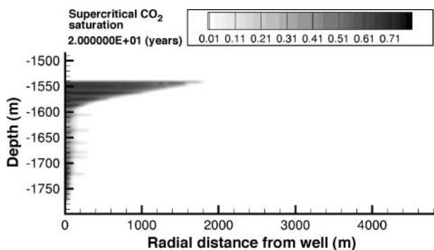
**Figure 21.** Saturation of supercritical CO<sub>2</sub> after 20 yr of injection into the Mount Simon Formation.
