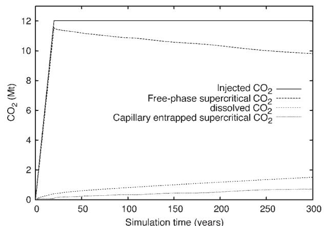
**Figure 19.** Mass balance of CO<sub>2</sub> injected into the Mount Simon Formation.
