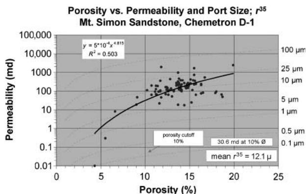
**Figure 11.** Plot of conventional core porosity versus permeability for Mount Simon Sandstone samples in the BASF Chemetron D-1 well, near Holland, Ottawa County, Michigan. Three probable spurious data points were excluded from the plot because of anomalously high permeability relative to porosity values.
