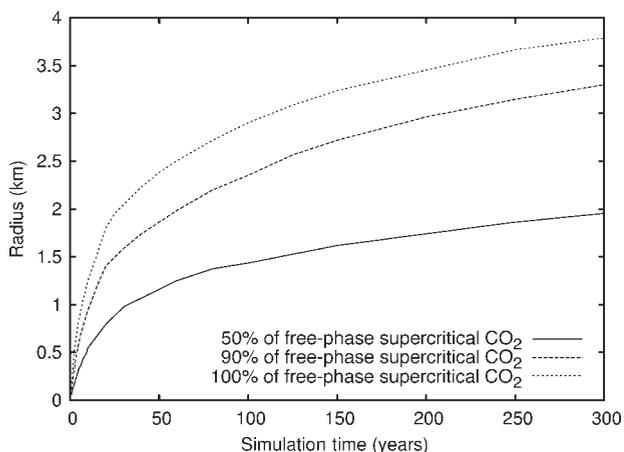
**Figure 20.** Distance and percentage saturation of the free-phase CO<sub>2</sub> injected into the Mount Simon Formation.
