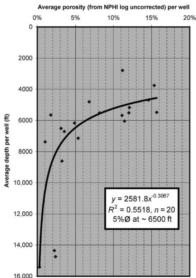
**Figure 10.** Plot of average measured driller's depth versus average, raw NPHI (uncorrected porosity) log. The trend line suggests that porosity decreases significantly below about 1981 to 2438 m (6500 to 8000 ft) in the Michigan Basin subsurface.
