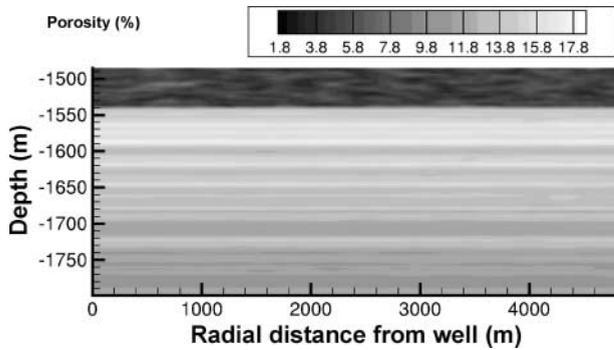
**Figure 15.** Geostatistical realization of diffusive porosity in the Mount Simon (1540–1799 m [5052–5902 ft]) and Eau Claire (1483–1540 m [4865–5052 ft]) formations.
